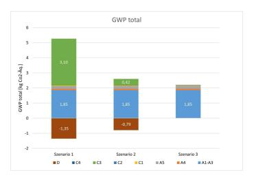
In scenario 1 (100 % energy recovery), "GWP total" is dominated by the production phase (modules A1A3) and waste treatment (module C3). The impacts within the system boundaries can be partially compensated by recovery potentials outside the system boundaries (Module D).
